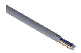
Quabbin control and signal cable, shielded, 15 conductors, 24 AWG, 7-stranded, tinned copper, PVC conductor insulation material, PVC jacket, gray, cut to length.
