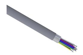
Quabbin control and signal cable, shielded, 10 conductors, 24 AWG, 7-stranded, tinned copper, PVC conductor insulation material, PVC jacket, gray, cut to length.
