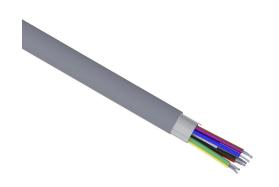
Quabbin control and signal cable, shielded, 9 conductors, 24 AWG, 7-stranded, tinned copper, PVC conductor insulation material, PVC jacket, gray, cut to length.
