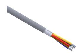
Quabbin control and signal cable, shielded, 8 conductors, 24 AWG, 7-stranded, tinned copper, PVC conductor insulation material, PVC jacket, gray, cut to length.
