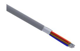
Quabbin control and signal cable, shielded, 7 conductors, 24 AWG, 7-stranded, tinned copper, PVC conductor insulation material, PVC jacket, gray, cut to length.
