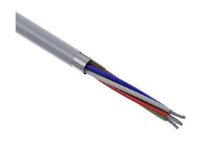
Quabbin control and signal cable, shielded, 6 conductors, 24 AWG, 7-stranded, tinned copper, PVC conductor insulation material, PVC jacket, gray, cut to length.
