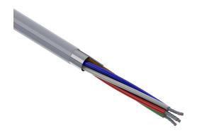
Quabbin control and signal cable, shielded, 6 conductors, 24 AWG, 7-stranded, tinned copper, PVC conductor insulation material, PVC jacket, gray, cut to length.
