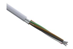
Quabbin control and signal cable, shielded, 5 conductors, 24 AWG, 7-stranded, tinned copper, PVC conductor insulation material, PVC jacket, gray, cut to length.
