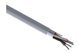
Quabbin control and signal cable, shielded, 4 conductors, 24 AWG, 7-stranded, tinned copper, PVC conductor insulation material, PVC jacket, gray, cut to length.
