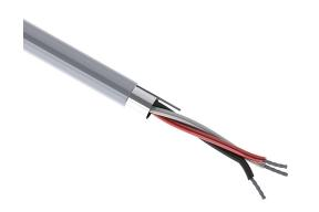
Quabbin control and signal cable, shielded, 3 conductors, 24 AWG, 7-stranded, tinned copper, PVC conductor insulation material, PVC jacket, gray, cut to length.
