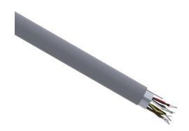
Quabbin control and signal cable, shielded, 8 twisted pairs, 24 AWG, 7-stranded, tinned copper, PVC conductor insulation material, PVC jacket, gray, cut to length.
