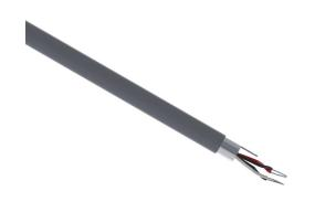
Quabbin control and signal cable, shielded, 2 twisted pairs, 24 AWG, 7-stranded, tinned copper, PVC conductor insulation material, PVC jacket, gray, cut to length.
