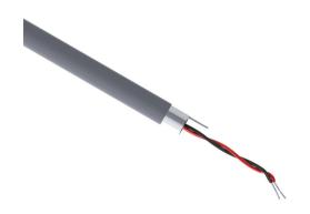
Quabbin RS-232 low capacitance data serial cable, shielded, 1 twisted pair, 24 AWG, 7-stranded, tinned copper, PVC conductor insulation material, PVC jacket, gray, cut to length.
