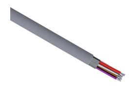
Quabbin control and signal cable, shielded, 15 conductors, 22 AWG, 7-stranded, tinned copper, PVC conductor insulation material, PVC jacket, gray, cut to length.
