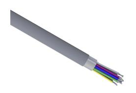
Quabbin control and signal cable, shielded, 12 conductors, 22 AWG, 7-stranded, tinned copper, PVC conductor insulation material, PVC jacket, gray, cut to length.
