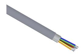
Quabbin control and signal cable, shielded, 10 conductors, 22 AWG, 7-stranded, tinned copper, PVC conductor insulation material, PVC jacket, gray, cut to length.
