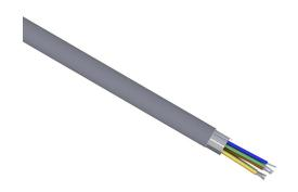
Quabbin control and signal cable, shielded, 8 conductors, 22 AWG, 7-stranded, tinned copper, PVC conductor insulation material, PVC jacket, gray, cut to length.
