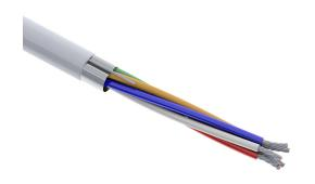
Quabbin control and signal cable, shielded, 6 conductors, 22 AWG, 7-stranded, tinned copper, PVC conductor insulation material, PVC jacket, gray, cut to length.
