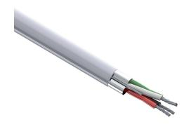
Quabbin control and signal cable, shielded, 4 conductors, 22 AWG, 7-stranded, tinned copper, PVC conductor insulation material, PVC jacket, gray, cut to length.
