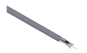
Quabbin control and signal cable, shielded, (1) shielded pair, (2) unshielded conductors, 22 AWG, 7-stranded, tinned copper, PVC conductor insulation material, PVC jacket, gray, cut to length.
