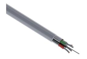
Quabbin control and signal cable, shielded, 2 twisted pairs, 22 AWG, 7-stranded, tinned copper, PVC conductor insulation material, PVC jacket, gray, cut to length.
