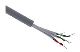
Quabbin serial cable, individual shielded, 3 twisted pairs, 22 AWG, solid, tinned copper, PVC conductor insulation material, PVC jacket, gray, cut to length.
