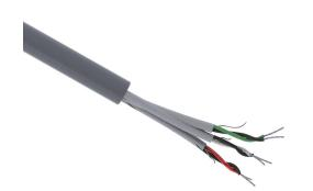
Quabbin serial cable, individual shielded, 3 twisted pairs, 22 AWG, solid, tinned copper, PVC conductor insulation material, PVC jacket, gray, cut to length.
