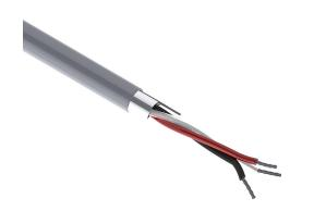
Quabbin control and signal cable, shielded, 3 conductors, 22 AWG, 7-stranded, tinned copper, PVC conductor insulation material, PVC jacket, gray, cut to length.
