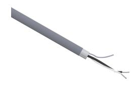
Quabbin control and signal cable, shielded, 2 conductors, 22 AWG, 7-stranded, tinned copper, PVC conductor insulation material, PVC jacket, gray, cut to length.
