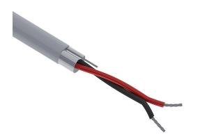
Quabbin control and signal cable, shielded, 2 conductors, 22 AWG, 7-stranded, tinned copper, PVC conductor insulation material, PVC jacket, gray, cut to length.
