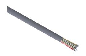
Quabbin control and signal cable, unshielded, 25 conductors, 22 AWG, 7-stranded, tinned copper, PVC conductor insulation material, PVC jacket, gray, cut to length.
