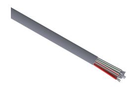
Quabbin control and signal cable, unshielded, 20 conductors, 22 AWG, 7-stranded, tinned copper, PVC conductor insulation material, PVC jacket, gray, cut to length.
