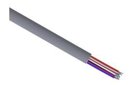
Quabbin control and signal cable, unshielded, 15 conductors, 22 AWG, 7-stranded, tinned copper, PVC conductor insulation material, PVC jacket, gray, cut to length.
