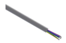
Quabbin control and signal cable, unshielded, 10 conductors, 22 AWG, 7-stranded, tinned copper, PVC conductor insulation material, PVC jacket, gray, cut to length.
