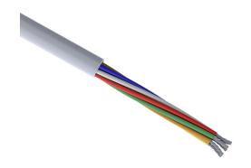
Quabbin control and signal cable, unshielded, 8 conductors, 22 AWG, 7-stranded, tinned copper, PVC conductor insulation material, PVC jacket, gray, cut to length.
