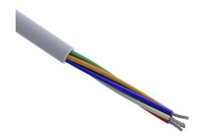
Quabbin control and signal cable, unshielded, 6 conductors, 22 AWG, 7-stranded, tinned copper, PVC conductor insulation material, PVC jacket, gray, cut to length.
