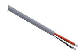
Quabbin control and signal cable, unshielded, 5 conductors, 22 AWG, 7-stranded, tinned copper, PVC conductor insulation material, PVC jacket, gray, cut to length.
