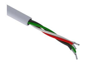
Quabbin control and signal cable, unshielded, 4 conductors, 22 AWG, 7-stranded, tinned copper, PVC conductor insulation material, PVC jacket, gray, cut to length.
