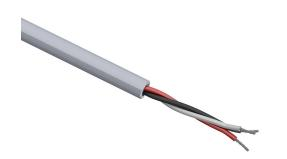
Quabbin control and signal cable, unshielded, 3 conductors, 22 AWG, 7-stranded, tinned copper, PVC conductor insulation material, PVC jacket, gray, cut to length.
