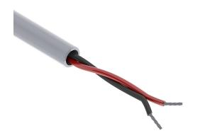
Quabbin control and signal cable, unshielded, 2 conductors, 22 AWG, 7-stranded, tinned copper, PVC conductor insulation material, PVC jacket, gray, cut to length.
