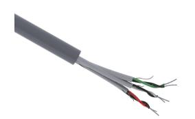
Quabbin serial cable, individual shielded, 3 twisted pairs, 20 AWG, 7-stranded, tinned copper, PVC conductor insulation material, PVC jacket, gray, cut to length.
