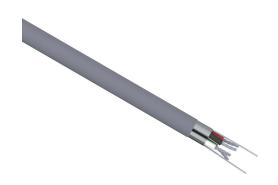
Quabbin control and signal cable, shielded, 2 twisted pairs, 20 AWG, 7-stranded, tinned copper, PVC conductor insulation material, PVC jacket, gray, cut to length.
