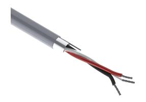
Quabbin control and signal cable, shielded, 3 conductors, 20 AWG, 7-stranded, tinned copper, PVC conductor insulation material, PVC jacket, gray, cut to length.
