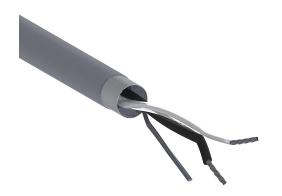
Quabbin control and signal cable, shielded, 2 conductors, 20 AWG, 7-stranded, tinned copper, PVC conductor insulation material, PVC jacket, gray, cut to length.
