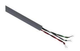
Quabbin serial cable, unshielded, 3 twisted pairs, 20 AWG, 7-stranded, tinned copper, PVC conductor insulation material, PVC jacket, gray, cut to length.
