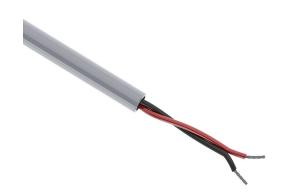
Quabbin control and signal cable, unshielded, 1 twisted pair, 20 AWG, 7-stranded, tinned copper, PVC conductor insulation material, PVC jacket, gray, cut to length.
