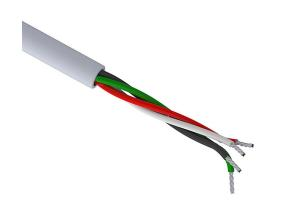
Quabbin control and signal cable, unshielded, 4 conductors, 20 AWG, 7-stranded, tinned copper, PVC conductor insulation material, PVC jacket, gray, cut to length.
