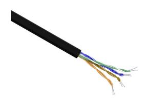
Quabbin Datamax flexible Cat5e industrial Ethernet cable, unshielded, 4 twisted pairs, 24 AWG, 7-stranded, tinned copper, HDPE conductor insulation material, PVC jacket, black, cut to length.
