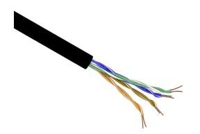
Quabbin Datamax Cat5e Ethernet cable, unshielded, 4 twisted pairs, 24 AWG, solid, bare copper, polyethylene conductor insulation material, PVC jacket, black, cut to length.
