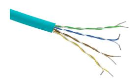
Quabbin Cat5e industrial Ethernet cable, unshielded, 4 twisted pairs, 22 AWG, solid, bare copper, polyethylene conductor insulation material, PVC jacket, teal, cut to length.
