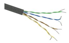
Quabbin Cat5e industrial Ethernet cable, unshielded, 4 twisted pairs, 22 AWG, solid, bare copper, polyethylene conductor insulation material, PVC jacket, black, cut to length.
