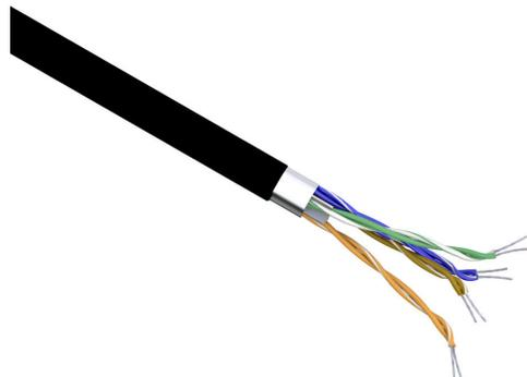
Quabbin Datamax continuous flexing Cat6/6a industrial Ethernet cable, shielded, 4 twisted pairs, 24 AWG, 7-stranded, tinned copper, HDPE conductor insulation material, polyurethane jacket, black, cut to length.
