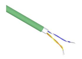
Quabbin Datamax continuous flexing Profinet cable, shielded, PLTC, ITC and AWM, 2 twisted pairs, 22 AWG, tinned copper, HDPE conductor insulation material, white, blue, yellow and orange, TPE jacket, green, cut to length.
