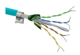
Quabbin continuous flexing Cat6/6a industrial Ethernet cable, shielded, 4 twisted pairs, 24 AWG, 7-stranded, tinned copper, polyethylene conductor insulation material, TPE jacket, teal, cut to length.
