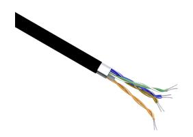
Quabbin Datamax continuous flexing Cat6/6a industrial Ethernet cable, shielded, 4 twisted pairs, 26 AWG, 7-stranded, tinned copper, HDPE conductor insulation material, polyurethane jacket, black, cut to length.
