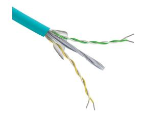
Quabbin continuous flexing Cat5e industrial Ethernet cable, unshielded, 2 twisted pairs, 24 AWG, 7/32-stranded, tinned copper, HDPE conductor insulation material, FR-TPE jacket, teal, cut to length.
